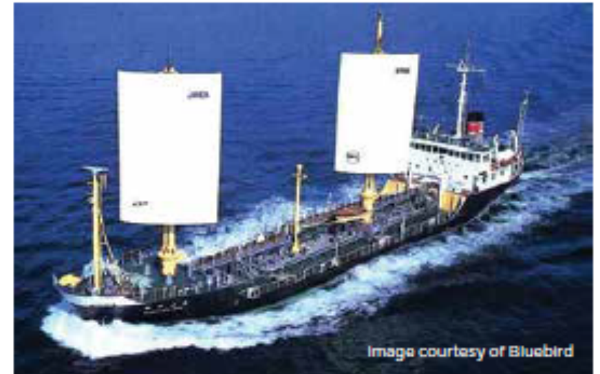
Vessel Shin Aitoku Maru with rigid sails
